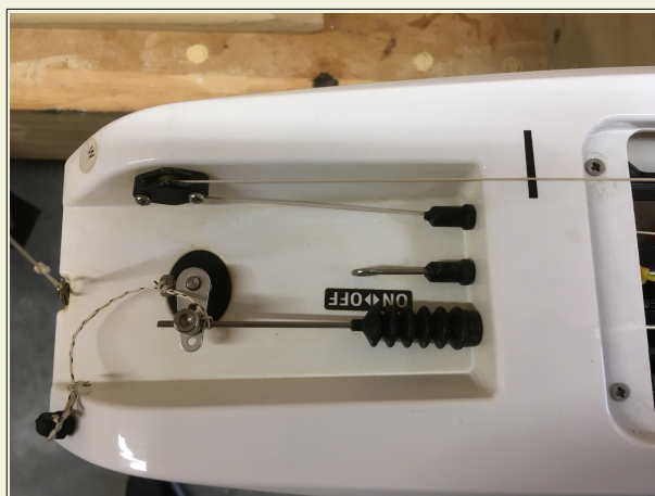
DF65 winch line clip position when sheeted in
