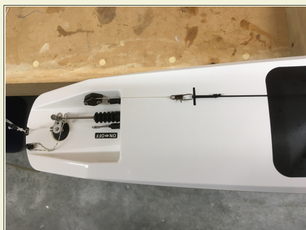
DF95 winch line clip position when sheeted in
