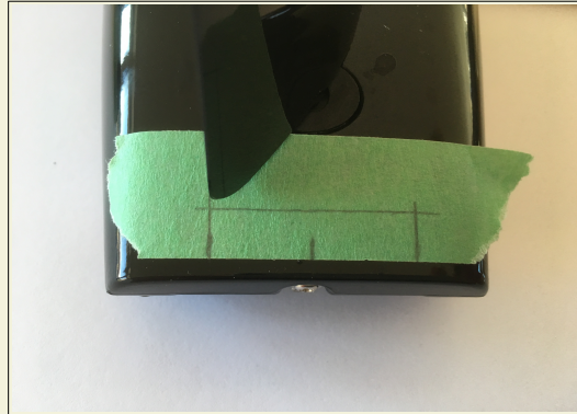
Setting max rudder throw to 35^\circ
