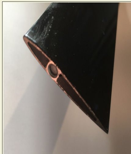
Keel extrusion cavities factory sealed
