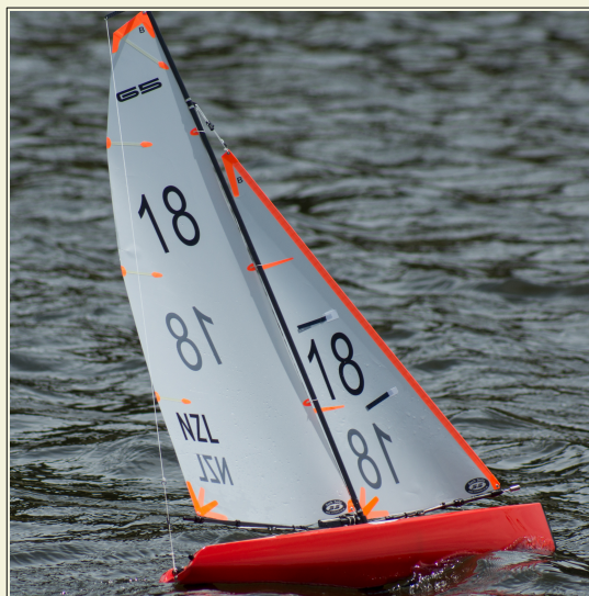
Twist – Note the changing angles of battens up both sails
