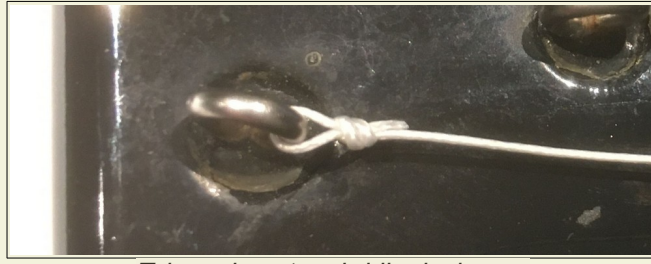
Tying a loop to a bridle deck-eye
